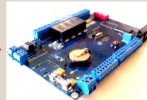
The **AT-INT** is one of our Asset Management Modules. It interfaces directly to MOD-LOG for the control and storage of Asset Events. It is essentially an RF Asset Tag Reader for our small and compact self powered **A-Tag**. These **A-Tags** are used in Asset Management, Process Tracking and Guard or personnel Tracking applications.
